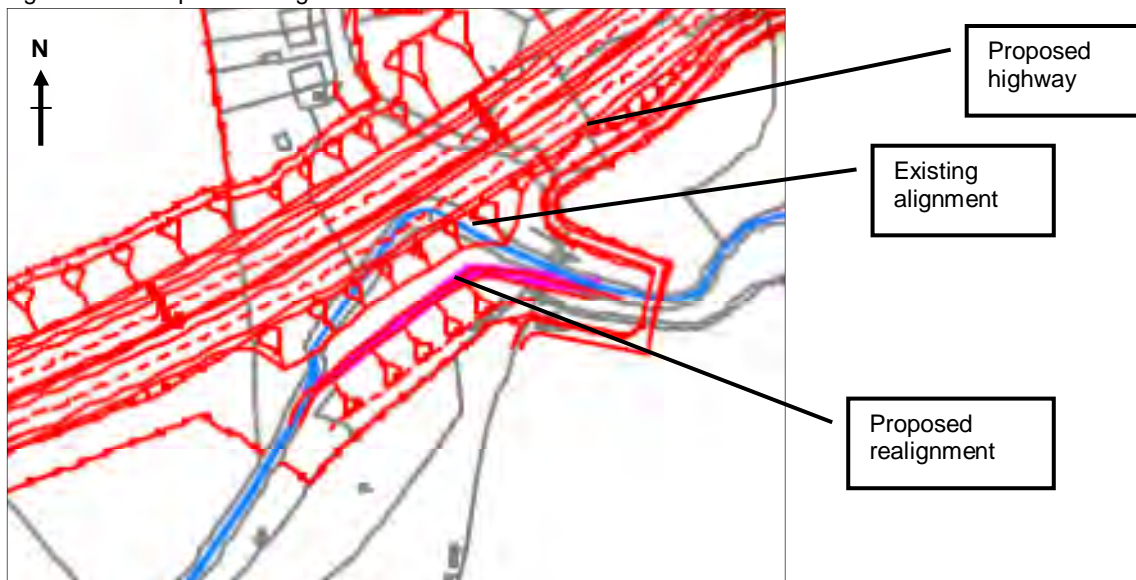
Figure B2.3: Proposed realignment at CH. 8830m.
